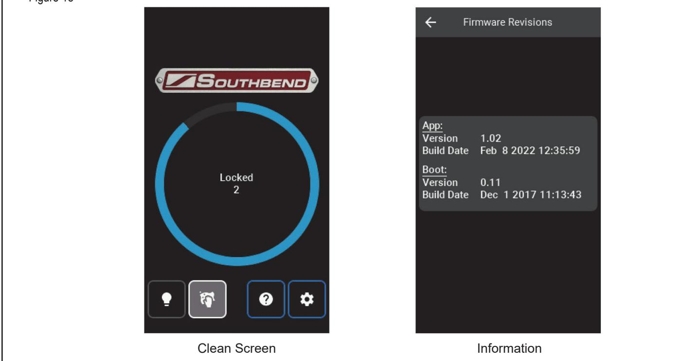
4. **Clean Screen** – Press and hold until the countdown wheel appears with countdown timer in the center of the screen. The screen will be locked for cleaning for 20 seconds. After blue wheel has completed circuit and countdown has reached 0, the screen will be accessible again.
