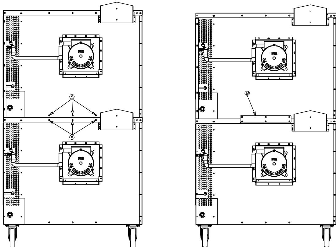
7. Insert two bolts (items "A" in the following diagram) up through the top of the lower oven and screw them into the threaded holes in the bottom of the top oven. Tighten these bolts and the screws that you did not tighten in the previous step.
