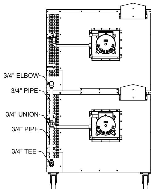
9. Install the flue stack as shown in the following diagram:
