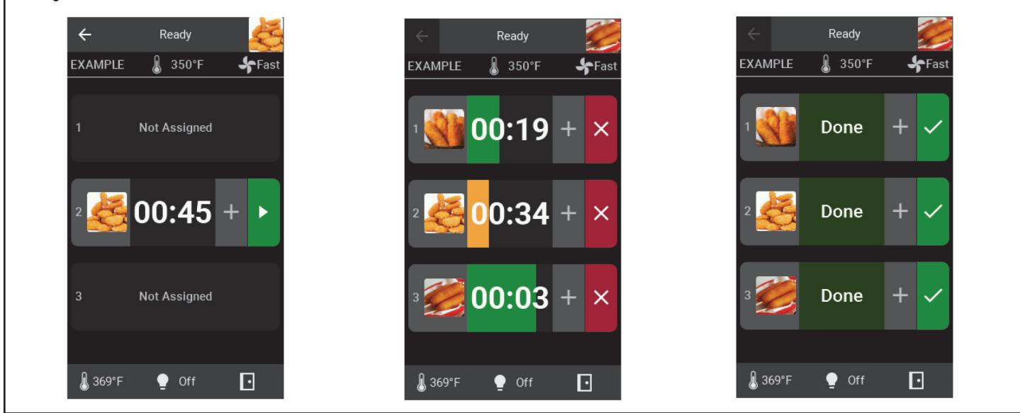
8. Choosing the start button will start the recipe and time can be added in one-minute increments. A progress bar depicts the time left. The bar starts as an amber indicator and changes to green at 20 seconds.
